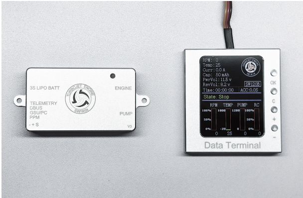
32 bit full digital ECU/Telemetry function GSU startup function
